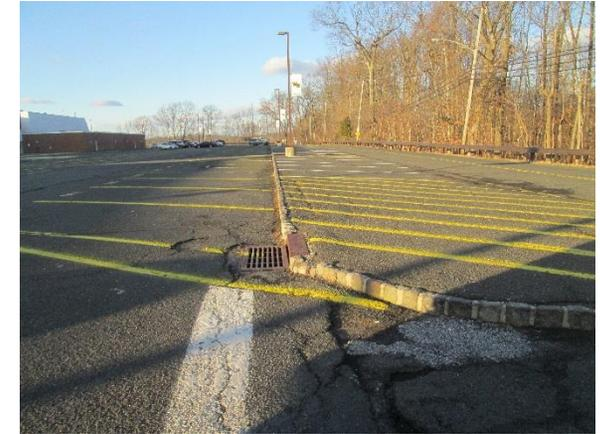
Rows of parking spots north and west of the school can be replaced with pervious pavement to provide stormwater being generated by the parking lots an opportunity to infiltrate. A preliminary soil assessment suggests that the soils have suitable drainage characteristics for green infrastructure.
